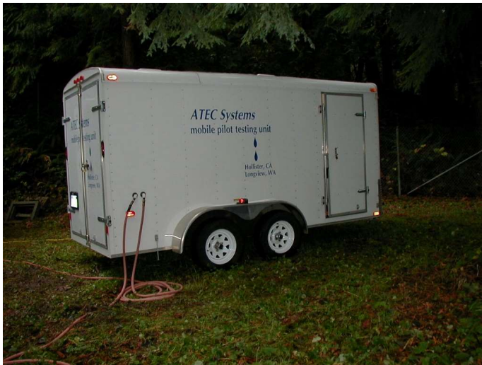
Figure(s) ATEC Iron and Manganese Removal Pilot Plant
